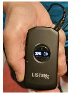
Whether you are using the hearing aid loop or the earpiece, you can adjust the volume using the UP/DOWN buttons on the front of the receiver.
